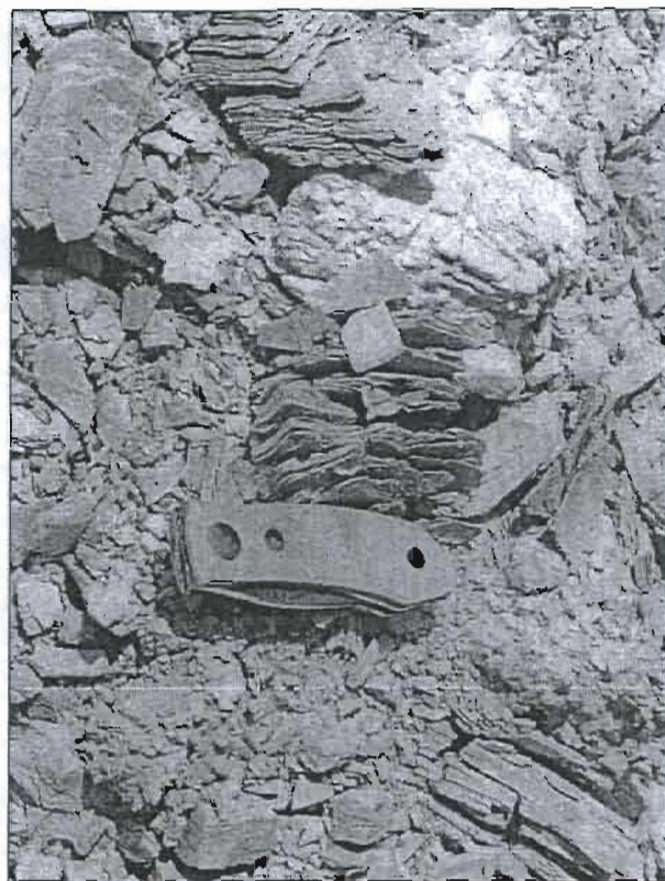
Figure 1. Foliate texture of high-magnesian attapulgite gelling-grade fuller's earth from the Florida–Georgia District near the axis of the Gulf Trough depositional embayment. This texture develops shortly after the raw clay is exposed for mining and is thought to be an indicator of high gelling strength. (Knife, for scale, is 10 cm long.)
