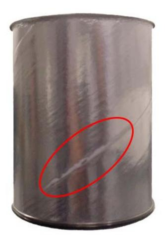
Table V – Defect No. 201, Not scorable. This photo shows label glue squeezing out at the overlap.
