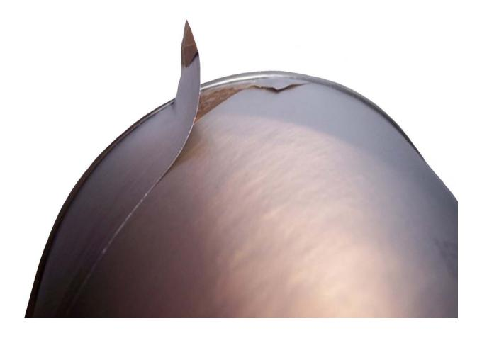
*Table V – Defect No. 208, Minor defect.* The label is not adhering to the body wall of the container.
