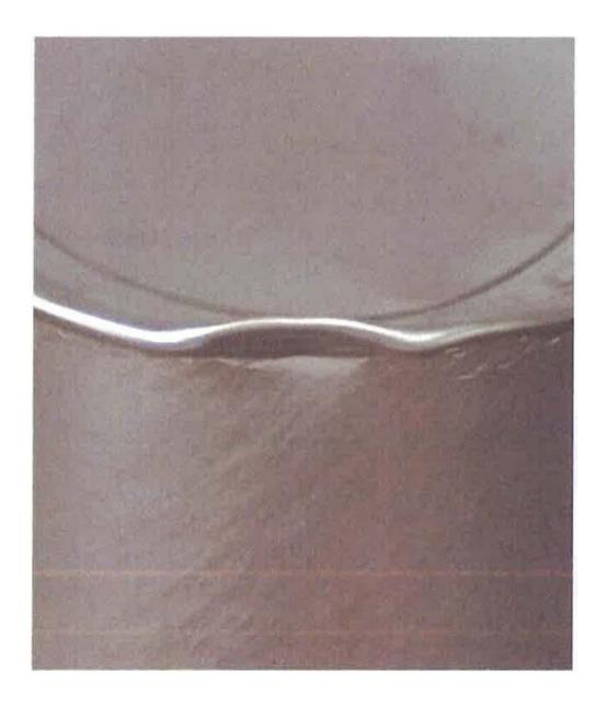
Table V – Defect No. 1, Critical defect. End is not completely connected to the composite container.
