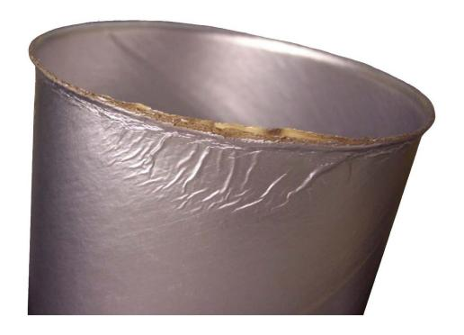
Table V – Defect No. 110, Major defect. Wet container materially affecting the usability of the product inside.
