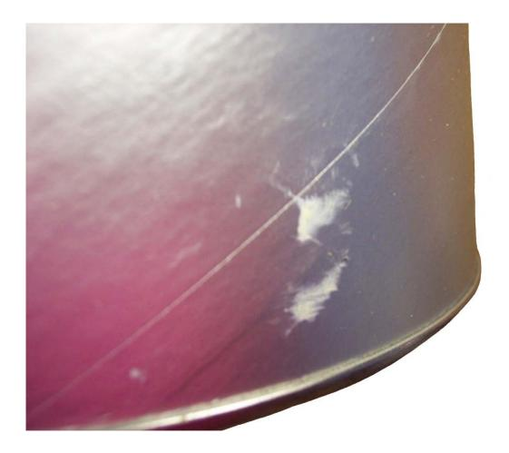
Table V – Defect No. 201, Minor defect. Any foreign material on the outside of the can other than glue from the label.
