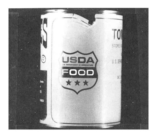
Table XI – Insignificant defect, Upper limit – not scored. Label torn or mutilated. If such a small tear obliterates any important text such as the ingredients or declared contents statement, the defect shall be classed as Defect No. 202 – Minor defect (nonmilitary purchases) or Defect No. 103 – Major defect (Military purchases).
