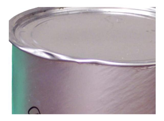
Table V – Defect No. 1, Critical defect. End is not completely connected to the composite container.
