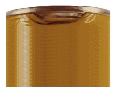
Table V – Defect No.1, Critical defect. End is not completely connected to the composite container.
